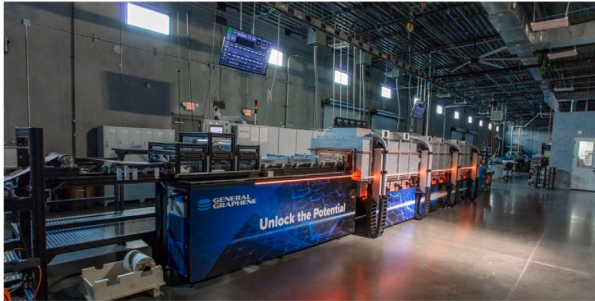
Fig. 4. General Graphene Inc. roll-to-roll graphene production line. Image credit: General Graphene.
